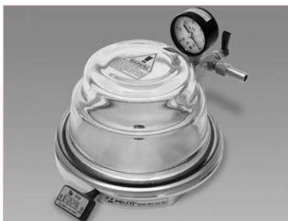
An inexpensive, miniature vacuum desiccator to warm embedding plastics while removing gas bubbles. The aluminium base is placed on a laboratory heating plate. The vacuum can be drawn through a porthole in the base plate. Suitable for use up to 120 °C, with a digital thermometer to measure plate temperature. Internal dimensions: 153 x 76 mm.
