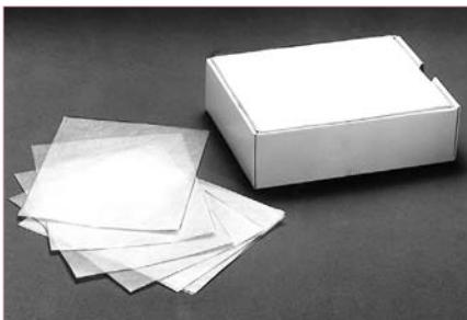
Square weighing papers with a glossy surface, suitable for weighing out powders.
