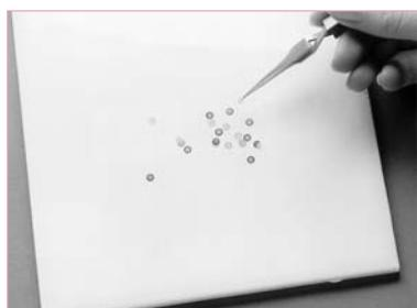
Easy to clean white tile, providing good background contrast for specimen manipulation.
