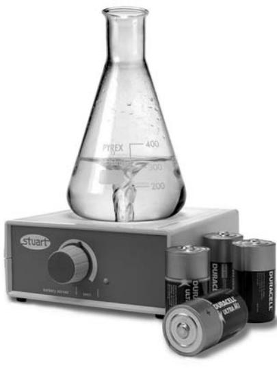
This portable stirrer is powered by long life batteries or mains power. It is ideal for use in incubators, glove boxes or in the field. Housed in a tough, chemically resistant ABS case, it is supplied complete with batteries and a 25 mm PTFE coated magnetic follower. It has variable speeds up to 1300 rpm with a stirring capacity of 1.5 litres.
