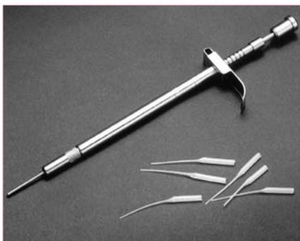
Slim micropipettes with excellent reproducibility, for use with very fine polyethylene capillary tips. These pipettes are ideal for dispensing gold sol preparations and particle dispersions. Available in two sizes, one with a working range of 1 - 10 µl in 1 µl increments, and the other with a range of 0.5 - 5 µl in 0.5 µl increments. Each pipette has a metal body with a stainless steel adjuster, for easy cleaning and sterilisation. A range of easy to fit replacement parts is also available.
