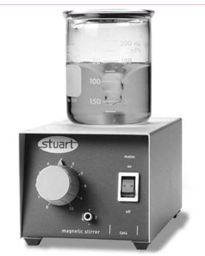
This compact magnetic stirrer has a clamp to accept a retort rod up to 16 mm in diameter. It has variable speed control up to 1300 rpm, with separate tuning controls for slow speed settings. It will stir volumes up to 1.5 litres and is supplied with one 25 mm long PTFE coated magnetic follower.
