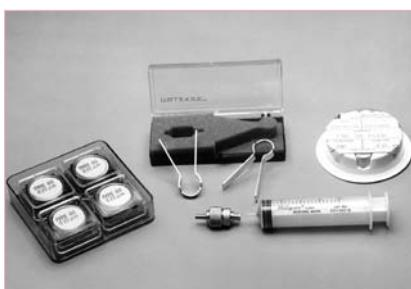
Millipore membrane filters are composed of biologically inert mixtures of cellulose acetate and cellulose nitrate. Available in a range of pore sizes.
